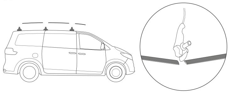
To create a level crossbar system, arrange legs and spacers as shown.
