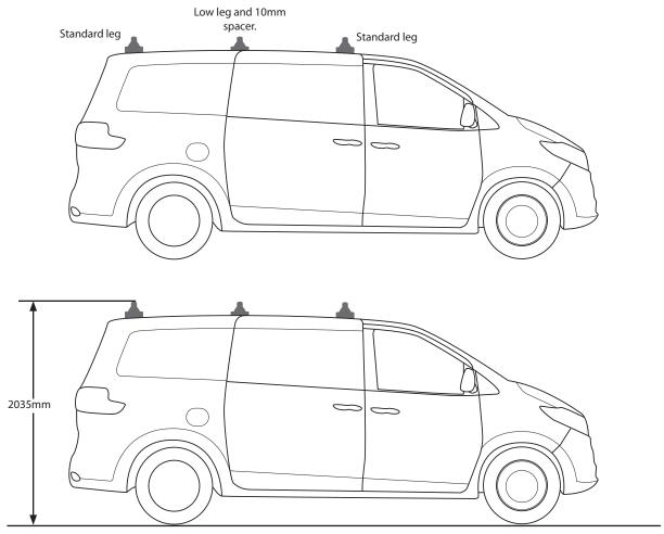
ATTENTION: Thoroughly check all fasteners are secure before driving away. Heights are for standard unloaded vehicles. Always check your specific vehicles height.
