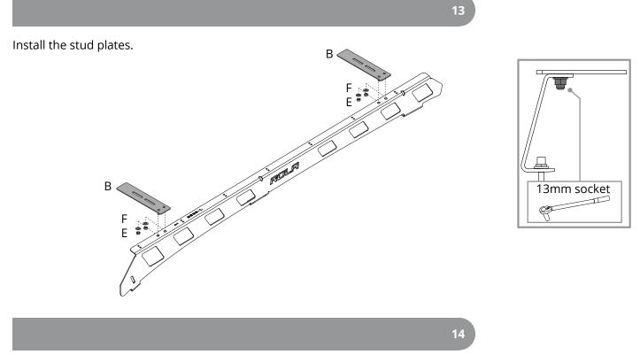
Install the assemblies into the roof.
