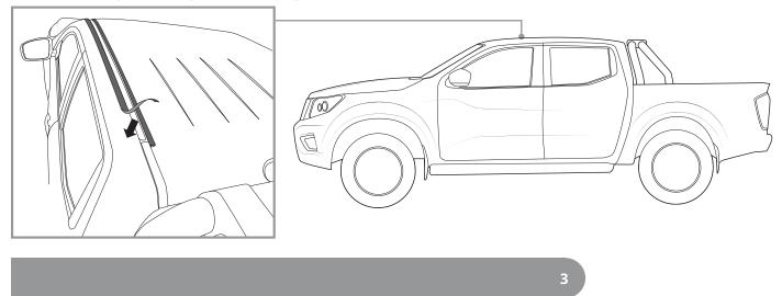
Place the Ridge Mounts into the ditch at the dimensions shown.
