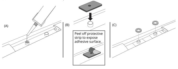
Assemble M8 hardware into the Ridge Mount Rails as shown.
