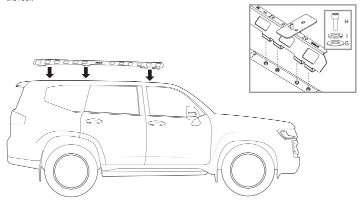
Tighten the M8 hardware with a 6mm allen key to 4-5Nm. Note: Access hardware through cutouts on side or holes located on top of the rail.
