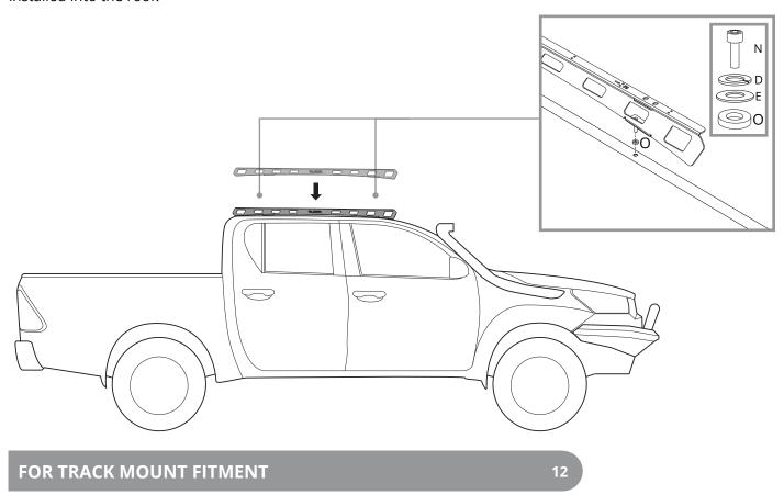
Drop the fitted square nuts into the accessory port on the pre-installed tracks of the vehicle.
