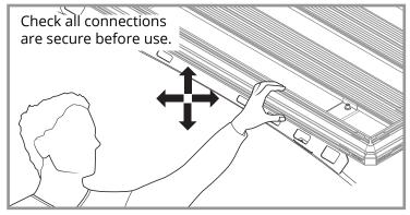
Wiring can be run and secured on the underside of the Ridge Mount rail as shown.
