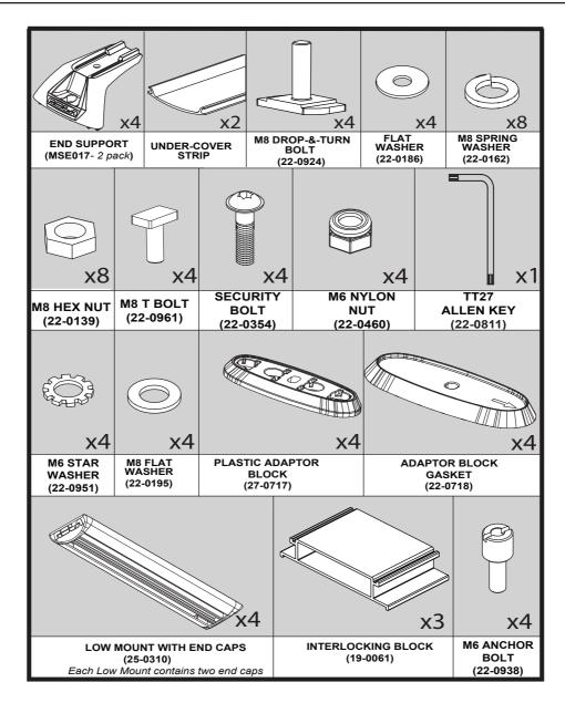
Prior to assembly, check that your roof rack kit contains all the parts as listed above. Ensure the vehicle roof is clean and dry.
