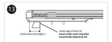
Cut the under-cover strip to the required lengths for each Low Mount.
