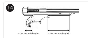
Cut the under-cover strips to the required lengths for each Low Mount.
