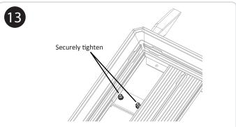
Tighten the fasteners on the top of the tray to secure the Low Mounts in place.
