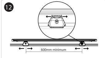
You can adjust the Low Mount to sit outboard, flush or inboard of the Titan Tray edge, depending on your preference and the distance between your vehicles roof rails.
