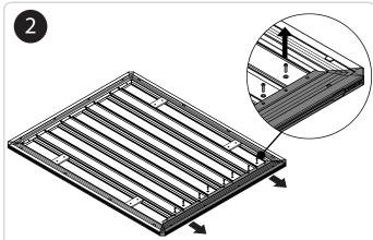
Place tray upside down. Remove fasteners on one side and remove the end plank.
