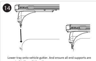
mounted in the vehicle gutter.
