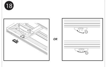
Insert under-cover strip lengths by sliding or clipping into the Low Mounts.
