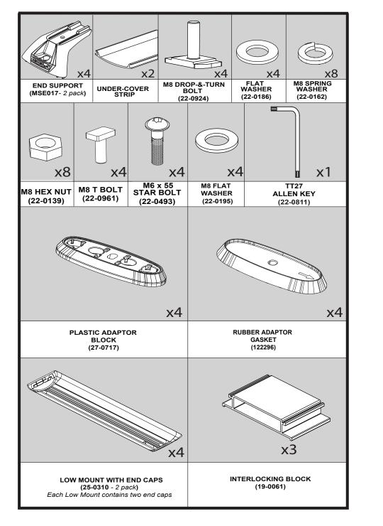
Prior to assembly, check that your roof rack kit contains all the parts as listed above.
