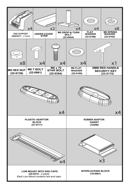
Prior to assembly, check that your roof rack kit contains all the parts as listed above. Ensure the vehicle roof is clean and dry.
