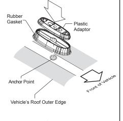
Select an Anchor Point from STEP 4 and with one of the supplied Rubber Gaskets place them over the top of the anchor point.
