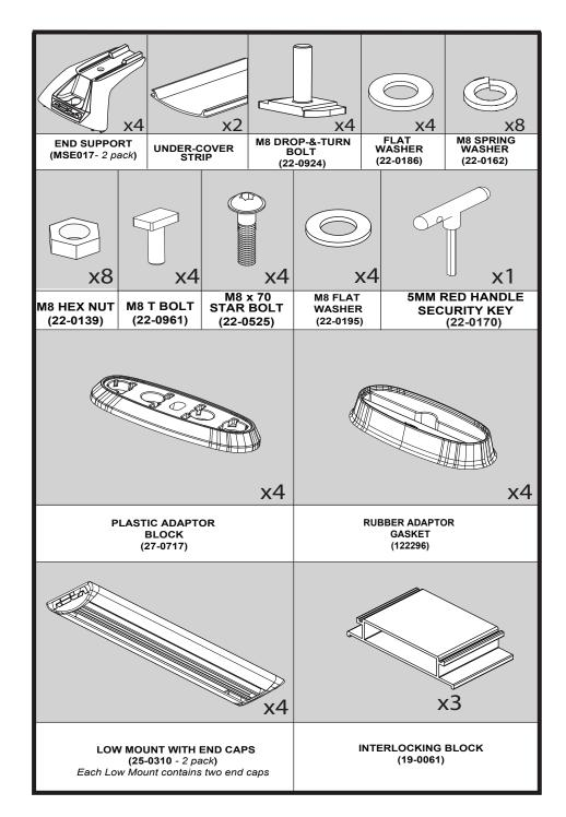
Prior to assembly, check that your roof rack kit contains all the parts as listed above. Ensure the vehicle roof is clean and dry.
